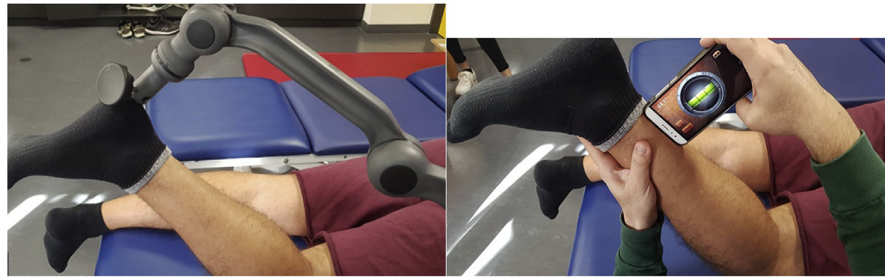
Fig. 3. Set up for the proprioception experiment, with subjects lying prone on an examination couch: (a) the plastic arm used as an indicator for memorizing the target angle through active knee flexion concentric repetitions, and (b) angle recording with the 'iHandy level' smartphone application, once the target angle (as perceived by participants) was reached.
