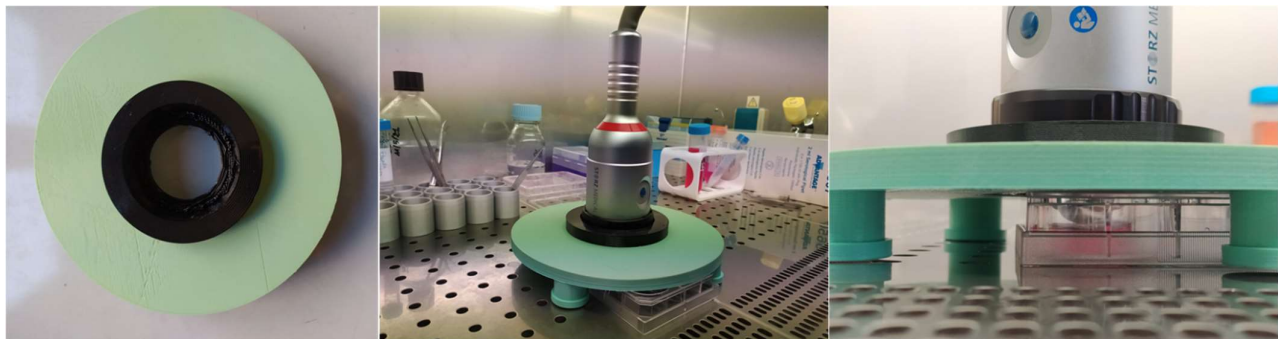
Figure 1. 3D-printed ESW cylindrical coil source support in PVC: the support is composed of two separate top parts (black, which adapts to the coil source size) and bottom parts (green, which keeps the support stable and suspended with respect to the 6-wellplates) were designed using Autodesk Fusion 360 (Autodesk, Inc., San Rafael, CA, USA) to minimize the loss of ESW energy at the interface between head of the device and the 6-multiwells.
