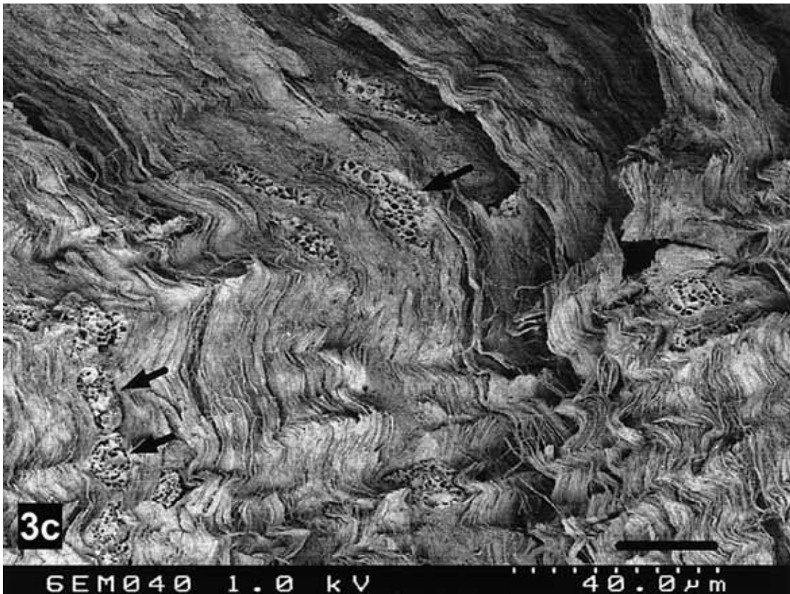
Fig. 3. Middle magnification of the same samples as in figure 5. a Lateral aspect of the sample with the border-deformed/undeformed fibers (dashed lines). Bar: 180 \mu\text{m} . b Middle of the indentation. Tangential layer (T) formed by fibers lying parallel to the cartilage surface. Fiber crimp in the the upper radial zone (arrows). Bar: 90 \mu\text{m} . c Fiber crimping in the center of the indentation at the border upper/lower radial zone. Chondrocytes (arrows) with segregation artifacts (due to ice crystal damage). Bar: 20 \mu\text{m} .
