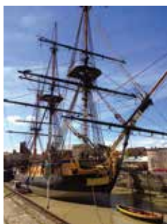
Fig 3: The sailing ship is the most widely used misrepresentation of a tensegrity structure.
